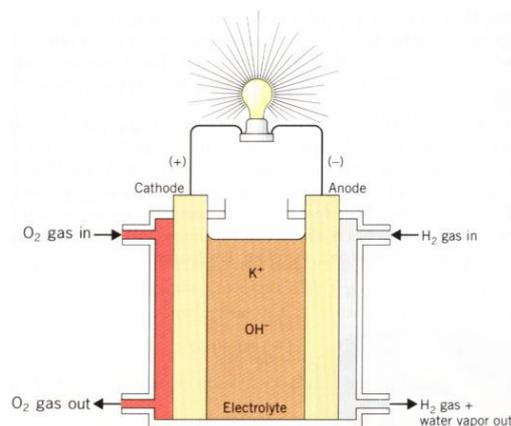
Fig 6.2 A hydrogen-oxygen fuel cell
