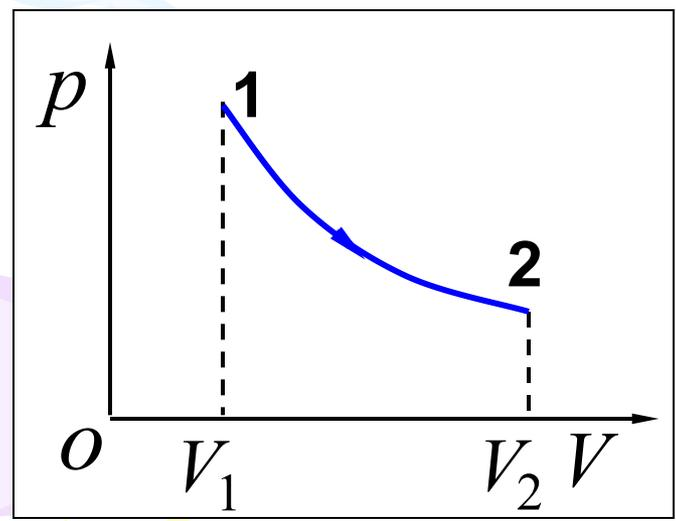
$$S_2 - S_1 = \int_1^2 \frac{dQ}{T} = \int_{V_1}^{V_2} \frac{m}{M} R \frac{dV}{V}$$
