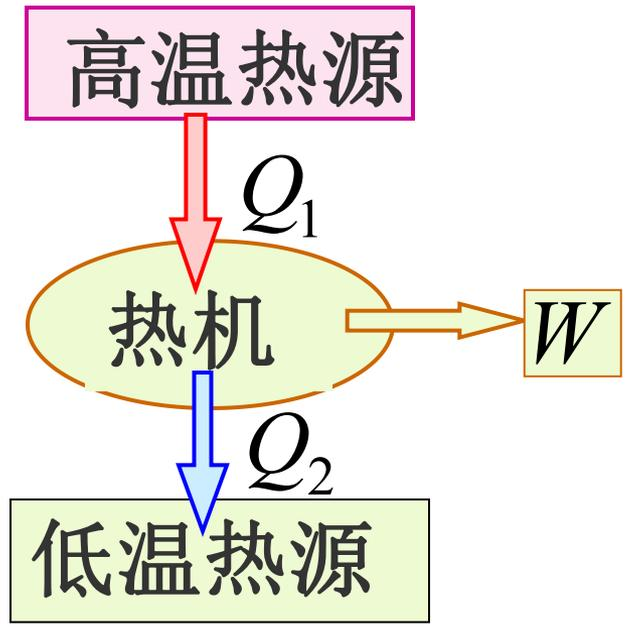
热机效率  $\eta = \frac{W}{Q_1} = \frac{Q_1 - Q_2}{Q_1} = 1 - \frac{Q_2}{Q_1}$
